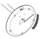
3 Tighten the 6 base bolt clockwise with the Allen wrench to secure column to base.
